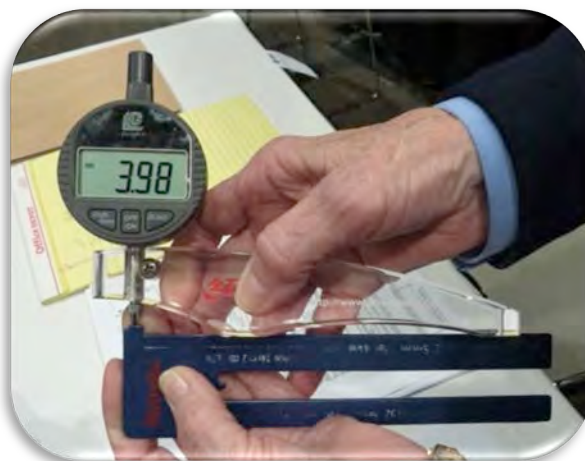
Figure 9: Easy method for checking the net gauge by using the digital thickness device
